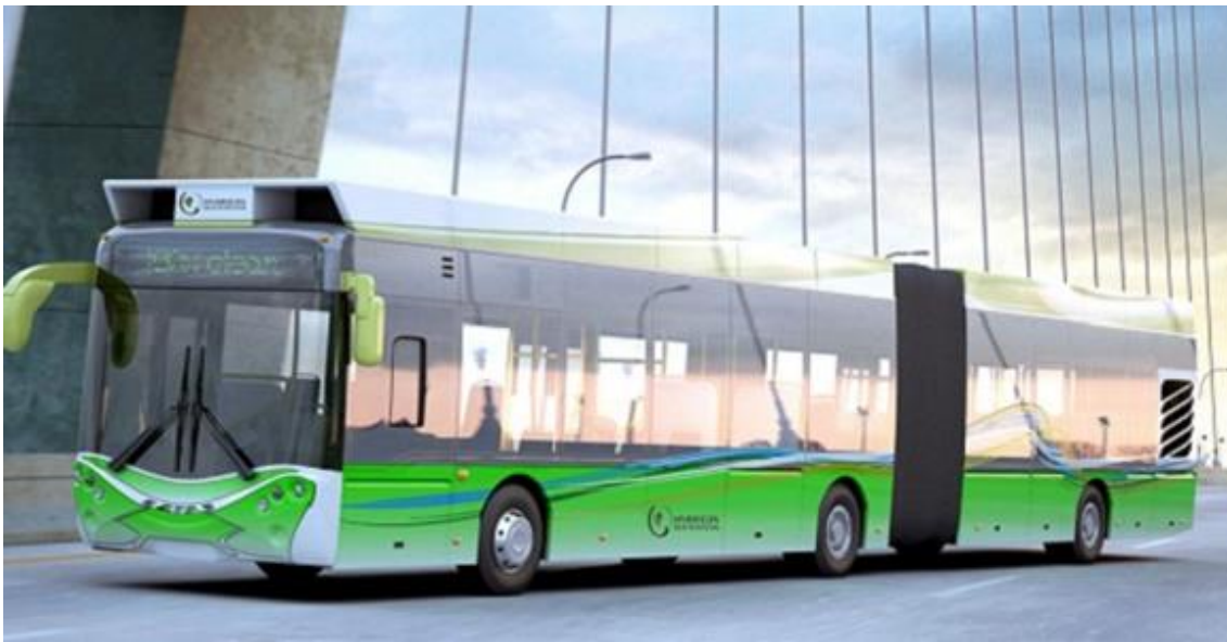
Figure 10B3: Ultra-fast charge all-electric articulated bus, 4 wheel-drive and 18 meters long
